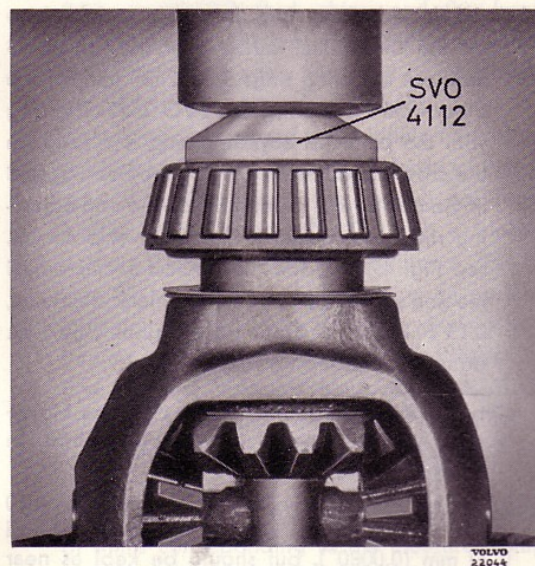
Fig. 54. Fitting the differential carrier bearing
